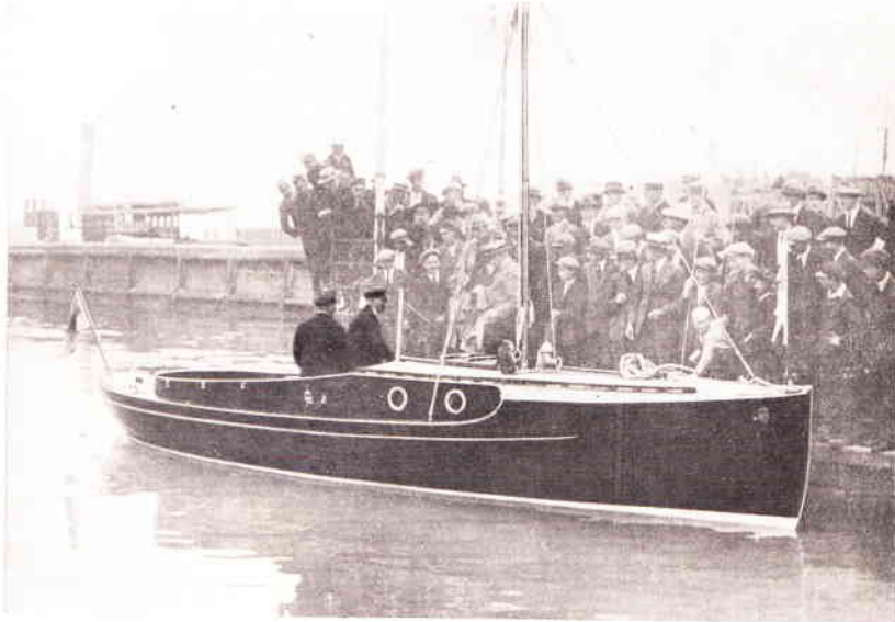
"Viking X" on her three months cruise round the coasts of Scandinavia. Data: Length: 9 metres. Beam: 2,15 metres. Depth: 0,8 metres. Weight: 3200 Kg. including a crew of 4 men. Speed: 7,2 knots. (See "The Motor Boat" of October 16th 1925.)
