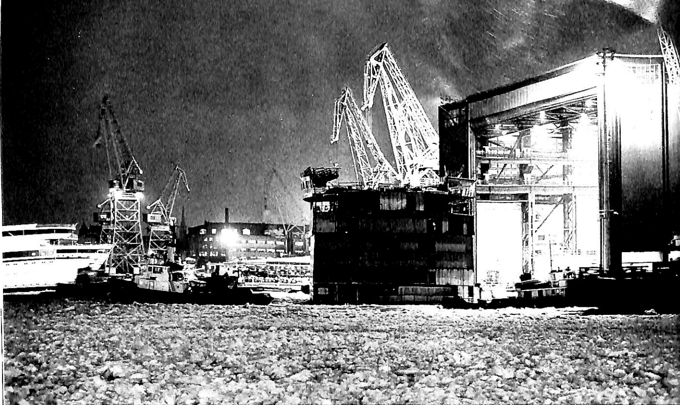
The ealier built mid-body is towed out from the building hall
